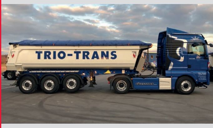
310673 MAN TGX XLX Euro 6c Thermomulden-Sattelzug / MAN TGX XLX Euro 6c Tipper semitrailer with thermal insulation „Trio-Trans“ (Bayern / Friedberg)
