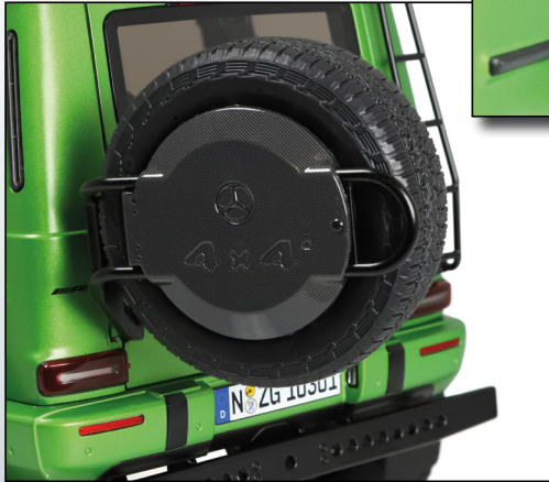
schwenkbarer Reserveradhalter / swivelling spare wheel holder
